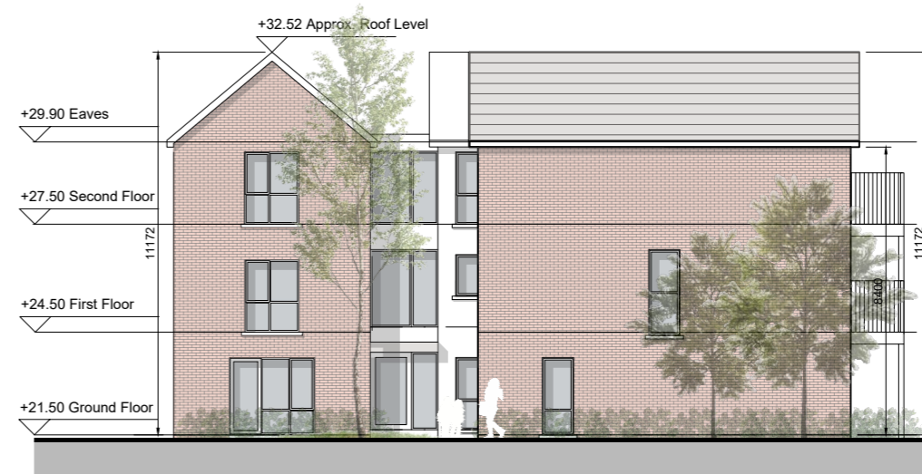
DUPLEX BLOCK B NORTH ELEVATION (REAR)
